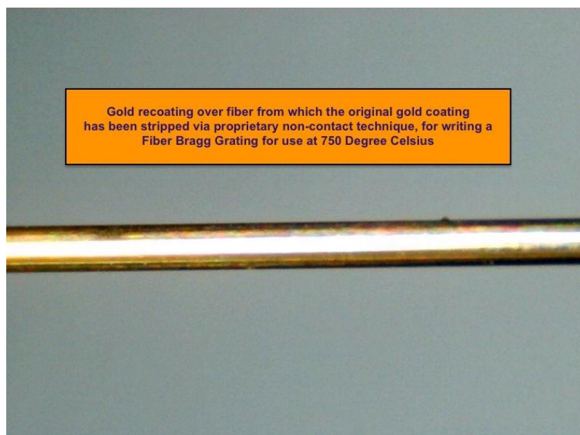
Fig.1 Schematic of a gold-coated FBG
