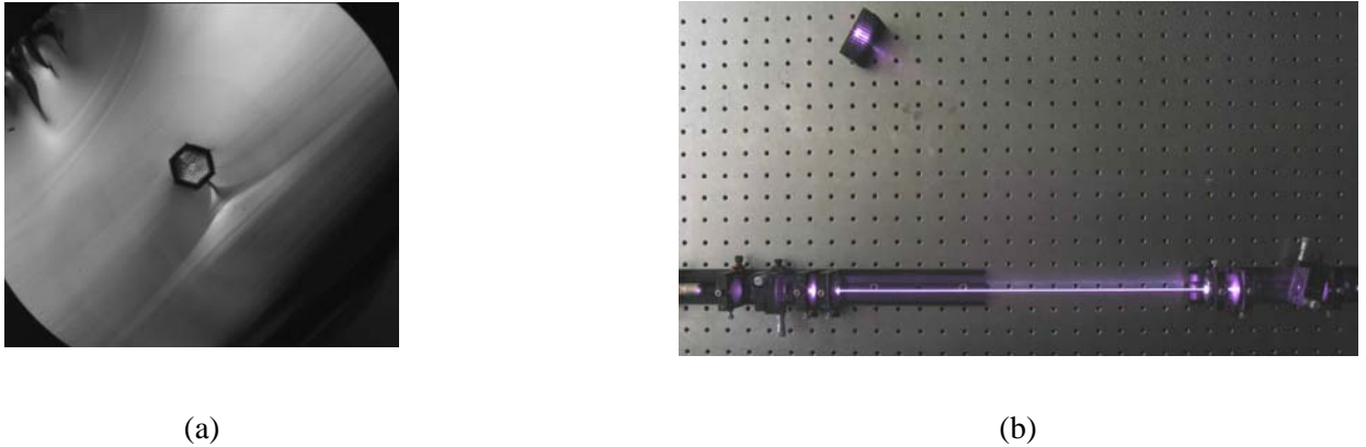
Fig. 8: (a) Microscope image of a rod-type photonic crystal fiber and (b) experimental setup of the rod-type fiber laser.
